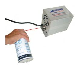
off the shelf refrigerant spray commonly found in electronics supply stores and also available from Xtreme. To simulate freezing conditions, spray the test port labeled on your heater where the thermostat control is located. By spraying this test port for 3 to 4 seconds, you can simulate the low temperature condition that will turn the heater
