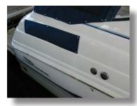
TIPS. A boat on a lift or a trailer will get much colder than a boat in the water. If you store your boat suspended on a lift, in addition to covering your bilge blower vents, you might wish to consider covering the outdrive unit. Alternatively, it may help to lower the boat into the water to keep cold air from circulating around the bottom of the boat, and allow the boat to extract heat from the water.
