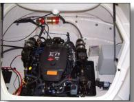
• **AVOID** mounting the heater to any tanks (water, gas, holding, etc), or any equipment such as the air conditioner, water heater, or generator. **AVOID** mounting the heater on or near any moving parts. These are pictures that illustrate unacceptable ways to mount your heater.
